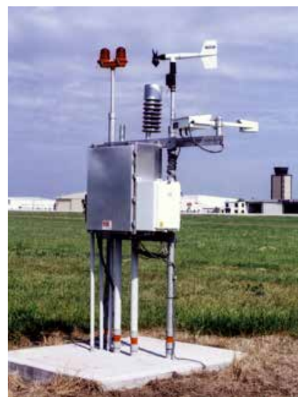
RWIS installed on an airfield – weather station with sensor suite (atmospherics)
